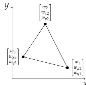
When solving  $A\bar{w} = \bar{f}$  one might want to impose different types of boundary conditions. Prescribing  $w(x_i) = 0$  for all  $x_i \in \mathcal{N}_h \cap \partial\omega$  is called *simply supported* boundary condition, whereas we refer to a *clamped* boundary condition when we additionally prescribe derivatives at each boundary vertex. The corresponding boundary masks should make use of the local to global mapping described above.
