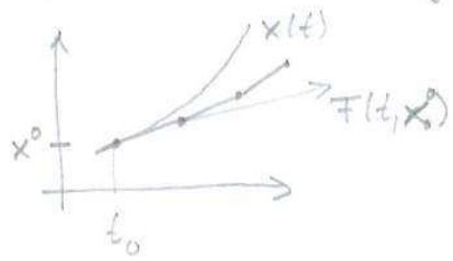
$$\phi_{t_0, t_0} x^0 \approx x^0 + (t - t_0) F(t_0, x^0)$$
