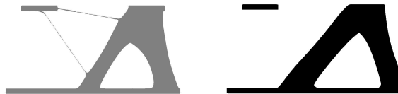
FIGURE 14. In the optimization of the excess probability for \eta = 0.4 decreasingly thin trusses are realized on the intermediate grey shape on the left until the left bearing is completely truncated via a topology optimization step (cf. Fig. 9 for the load configuration). The final result is shown on the right. (Figure reprinted from [24, Fig. 7])
