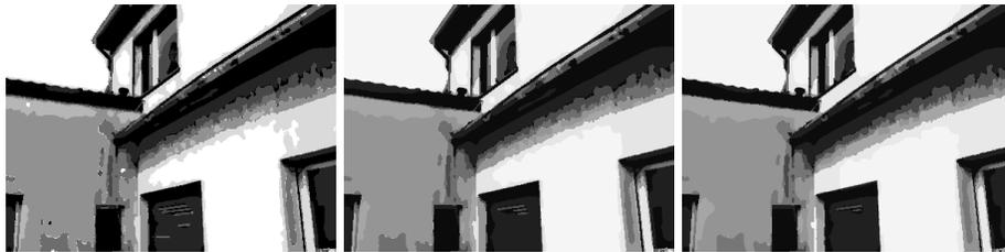
**Fig. 4.** Intermediate results of the segmentation in eight segments shown in Figure 3 after 50 (left), 250 (middle) and 700 (right) gradient descent steps.
