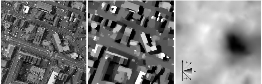
Joint denoising and anisotropy estimation: original image, anisotropic cartoon and estimated orientation.
