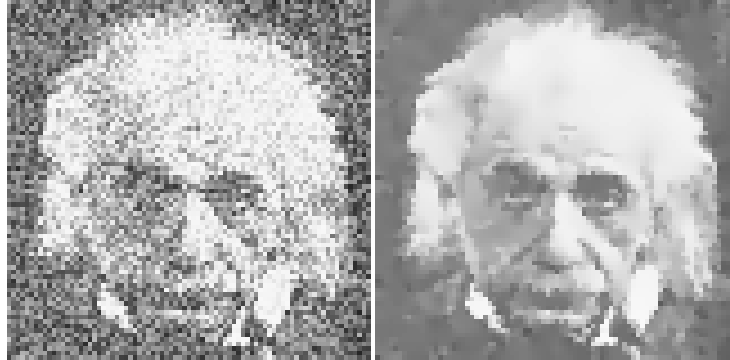
Figure 2: The noisy image on the left is successively smoothed by nonlinear diffusion. On the right the resulting smoothed image with enhanced edges is shown.
