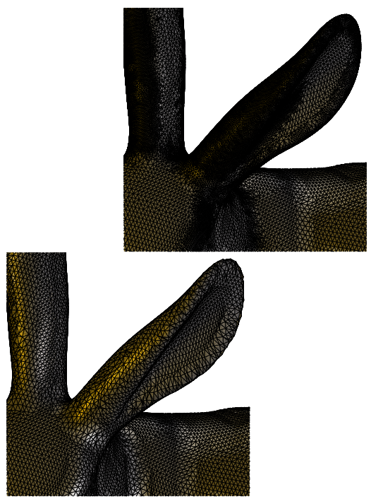
Figure 9: The resulting surface mesh (top) from an adaptive algorithm is compared with the corresponding grid of an evolution with fixed triangulation (bottom). The areas of high curvature are clearly visible as refinement regions.
