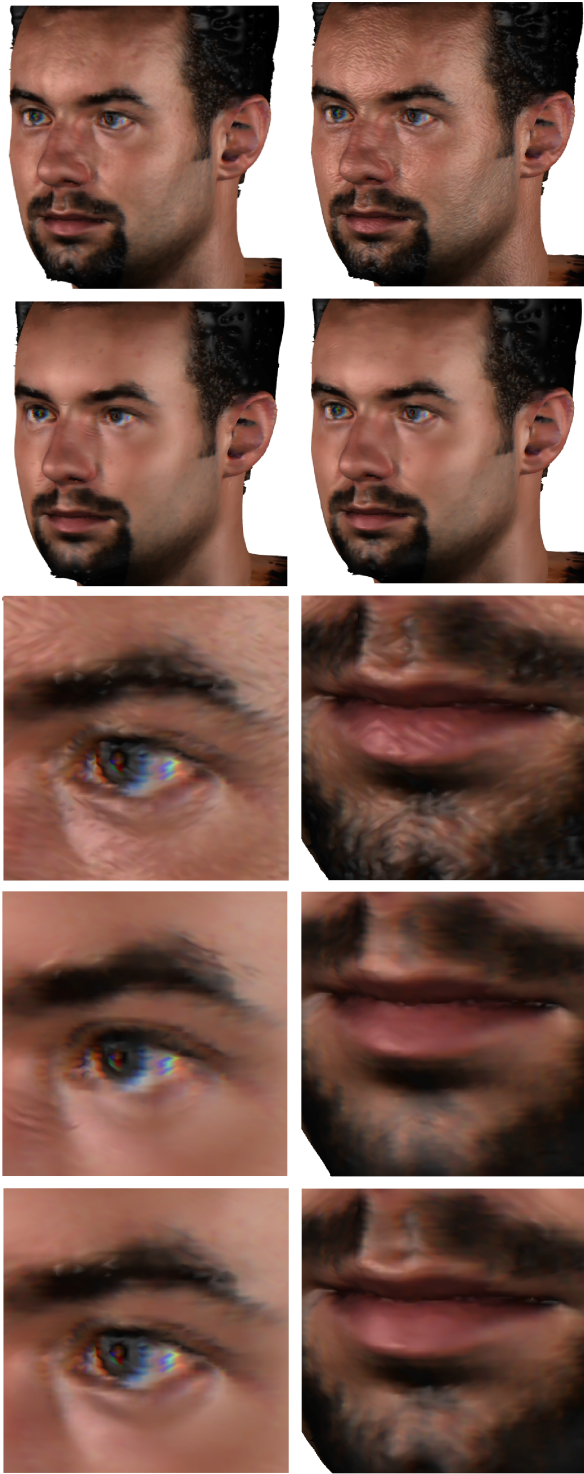
Fig. 7. A surface obtained from a laser scan with an onscribed photographic texture (top left) and the same surface with moderate superimposed, isotropic noise (top right) are depicted. The latter one is considered as initial surface for the combined geometry and texture evolution. In the second row we compare results of the pure geometry evolution (left) and the combined model (right). Furthermore, two areas with characteristic differences are magnified (on the remaining left column the left eye and on the right column the mouth region). In the third row the original noisy subregions are shown, whereas in the fourth and fifth row we have depicted magnified results of the pure geometry evolution and the combined evolution, respectively. Always the same evolution timestep t = 0.00012 is considered.
