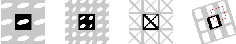
FIGURE 2. From left to right the different cells with different type of perforation are displayed: cells with single ellipsoidal holes, cells with  $2 \times 2$  ellipsoidal holes, cell structures consisting of axes aligned and diagonal trusses, freely rotated cells with rectangular holes representing orthogonal trusses (see red marking).
