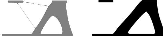
Figure 7: In the optimization of the excess probability for \eta = 0.4 decreasingly thin trusses are realized on the intermediate grey shape on the left until the left bearing is completely truncated via a topology optimization step (cf. Fig. 4 for the load configuration). The final result is shown on the right.
