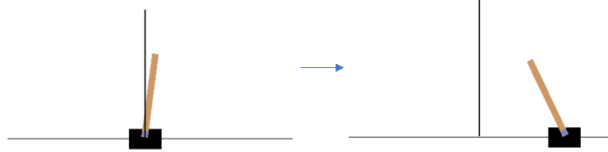
Figure 4.7: A representation of the cart-pole problem. Applying the action 1 pushes the cart to right. The agent must then react properly so to preserve the pole equilibrium.
