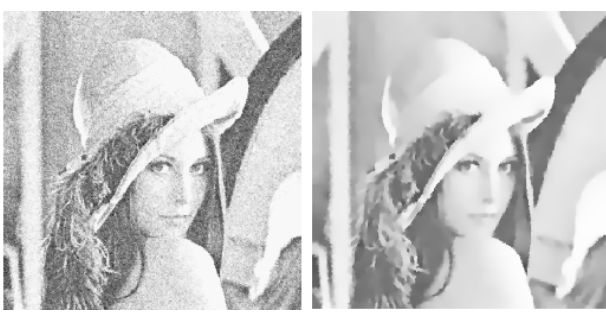
Figure 2: The noisy image on the left is successively smoothed by nonlinear diffusion. On the right the resulting smoothed image with enhanced edges is shown.
