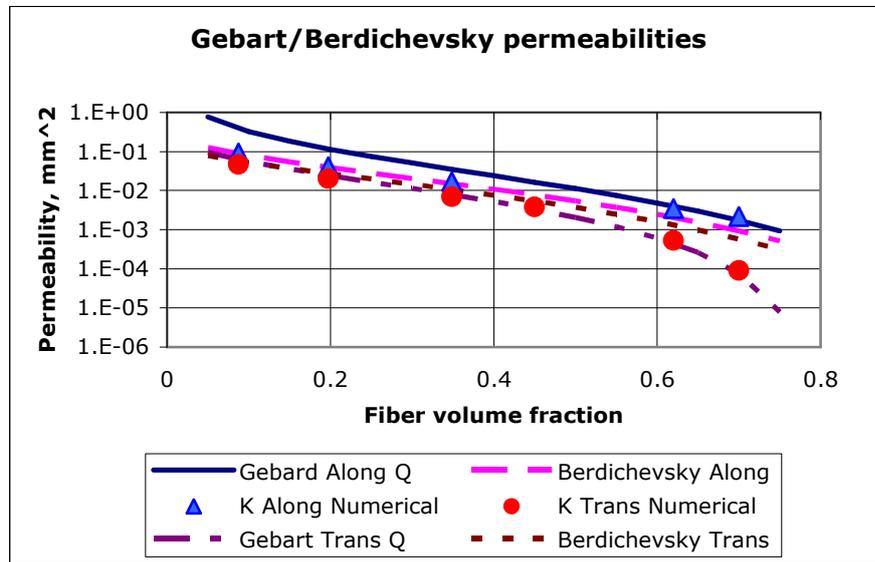
Fig. 2 Comparison of the Gebart/Berdichevsky formulas with numerical results
