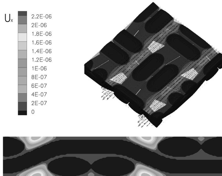
Fig. 3. 3D image and a 2D cut of the calculated flow field in the Natte model
