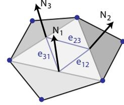
segments connecting these midpoints. Indeed, fixing a triangle  $T$  with edges  $e_1, e_2, e_3$  and corresponding edge normals  $N_1, N_2, N_3$  we find that  $dN(e_{ij}) = \int_{e_{ij}} dN = N_j - N_i$ , where  $e_{ij}$  is the line segment connecting the midpoint of  $e_i$  with that of  $e_j$ . Using the vector identity  $e_k = -2e_{ij}$ , where  $k$  is the complementary index to  $i$  and  $j$  in  $T$ , we accordingly define
