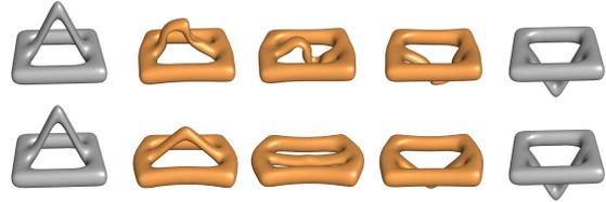
**Figure 9:** Discrete geodesic for low (top,  $\eta = 0.005$ ) and high (bottom,  $\eta = 0.1$ ) bending resistance ( $\lambda = \mu = 1$ ). Stiff materials prefer the handle being folded (inducing bending dissipation) whereas soft materials stretch the outer frame (i.e. induce tangential distortion) to avoid folding.
