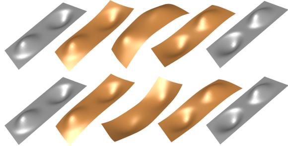
**Figure 5:** Symmetric setups can lead to non-unique geodesic paths. The flat plate as an intermediate shape is avoided since it would induce high tangential distortion. Therefore the bumps flip to the other side successively, while the order of flipping does not effect the accumulated dissipation.
