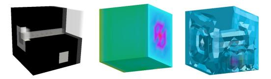
Figure 4: Cut-open unit cube with different diffusion regions, initial isosurfaces of ion concentration and final isosurfaces of ion concentration after 10 time units.
