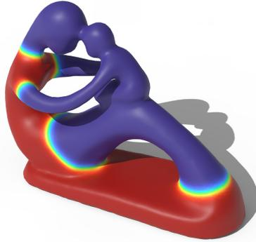
Figure 9: Distortion minimizing segmentation of the ‘fertility’ model (courtesy of the AIM@SHAPE project). Interface width is given by  $\varepsilon = 0.02$  and the distortion weight by  $\omega = 0.1$ . For this example, minimizing (13) yields segment boundaries following paths with negative Gauß curvature.
