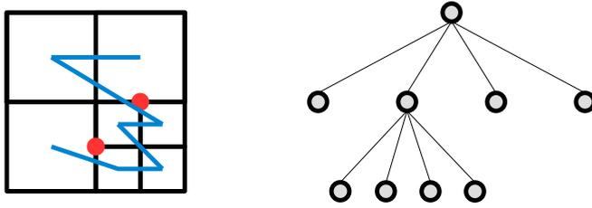
**Fig. 1.** Simple example for a two-dimensional quadtree grid (left) with the corresponding tree (right) and the discrete iterate of the Morton curve that can be used to linearize the tree (blue). Hanging corners of the adaptive grid are marked in red.
