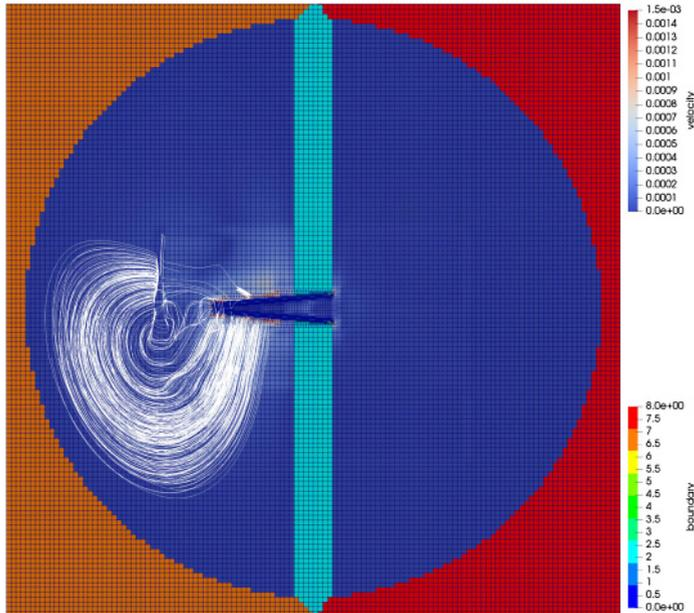
**Fig. 7.** Velocity field of the simulated electro-osmotic flow in the charged pore system.
