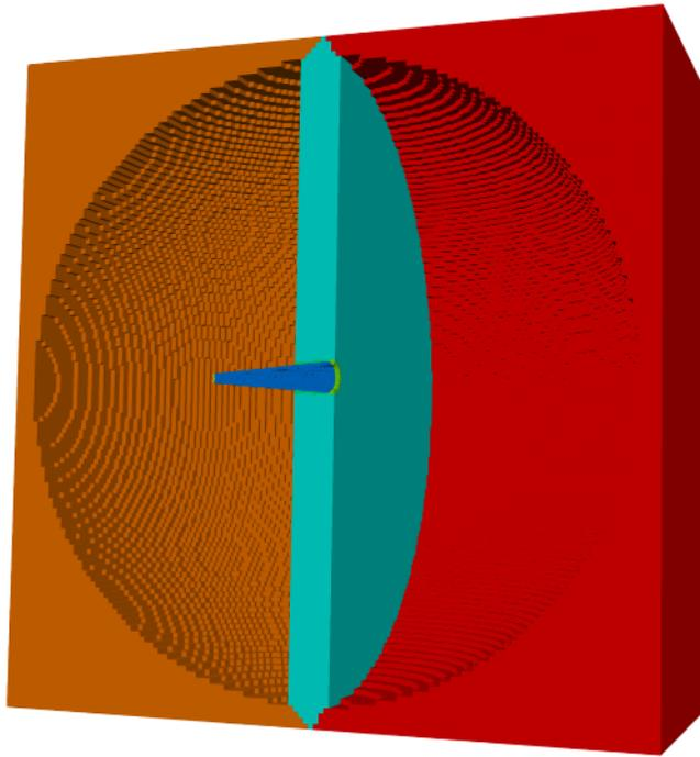
**Fig. 6.** Simulation setup of a charged pore. We charge the body of the capillary (royal blue) and apply an electric field by setting a potential at the hemispheres (orange and red) to obtain an electro-osmotic flow around the pore.
