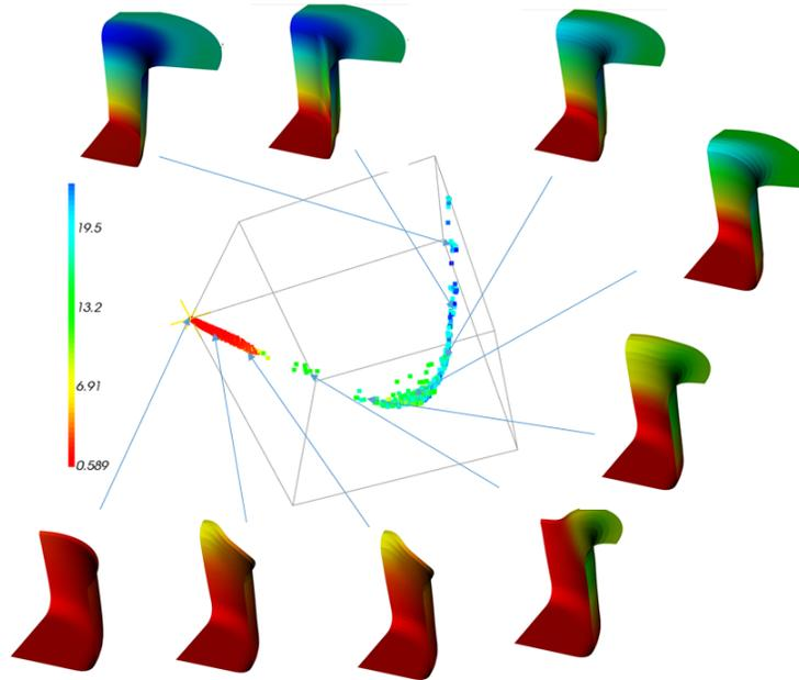
**Fig. 2** Representation of a simulation ensemble in a 3D space of the projection coefficients. Each point represents a shape at the end of the forming process. The points are colored by a simulation parameter and the color coding of the shapes correspond to the deformation differences to a reference simulation, where red indicates zero difference. Two groups are of interest, one “straight” cluster on the left hand side and an elongated curved cluster from the middle to the right hand side.
