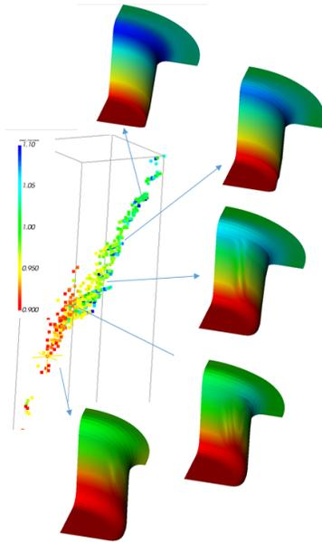
**Fig. 3** Latent representation of the 3D deformations (mesh functions  $x$ ,  $y$  and  $z$ ) showing a relation to the thickness (color of the points). The color on the shape shows the differences to a reference shape.
