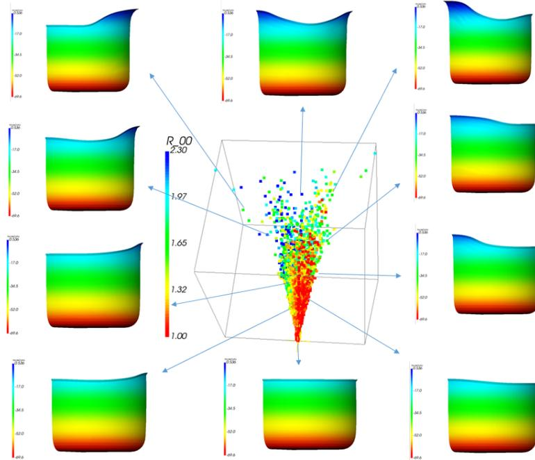
**Fig. 5** Representation of a cluster where each point represent a shape at the end of the forming process. The points are colored by the input parameter  $R_{00}$  and the color coding of the shapes correspond to the deformation differences in direction  $z$  to a reference simulation, where red indicates zero difference.
