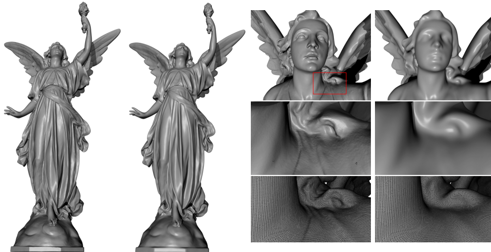
Fig. 4.3: Mean curvature motion is applied to the Lucy statue. On the left the initial surface and the result after 19 time steps with time step size \tau = 0.0004 are shown. On the right, we render corresponding blow ups at two different scales and overlay the finest scale blow up with the mesh generated using the marching cubes algorithm [39].
