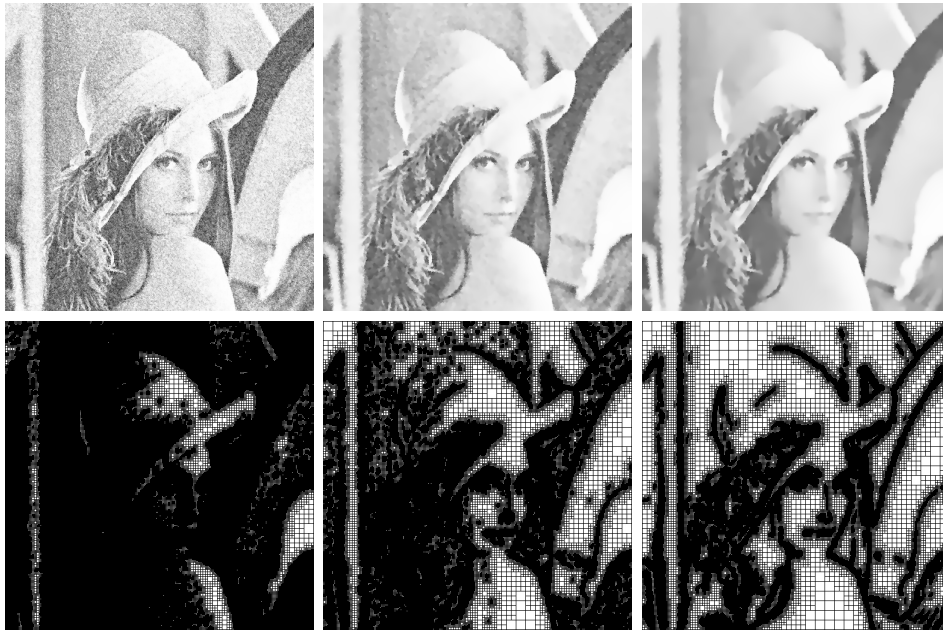
FIG. 3. From left to right several timesteps of the selective image smoothing on adaptive grids are shown.
