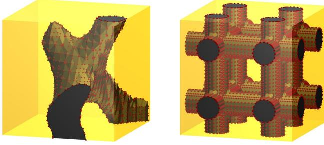
FIG. 4.2. *Virtual nodes on part of a trabecular aluminum structure at resolution  $17^3$  and an artificial rod dataset at resolution  $33^3$  are depicted as little red spheres. For the construction of the local auxiliary mesh,  $\gamma$  has been approximated by  $\gamma^\boxtimes$  and thus appears non-smoothly shaded in the image. The underlying uniform hexahedral mesh and the location of virtual nodes on its edges and some of its diagonals is clearly visible from the left picture.*
