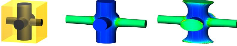
FIG. 7.3. For a  $1 \times 1 \times 1$  rod dataset, the difference between periodic (middle) and Dirichlet (right) boundary conditions is shown for one tensile loading case. Dirichlet boundary conditions prevent the longitudinal rods from thinning at the boundary and force the transverse rods to an elliptic cross section at the boundary, leading to higher average stress for the same macroscopic strain. Color encodes the von Mises stress at the interface.
