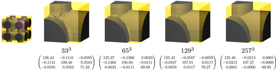
FIG. 7.2. For  $2 \times 2 \times 2$  rods of diameter/length ratios 0.38, 0.33, 0.24 (left), we show a zoom to one trabecular crossing at different computational resolutions ranging from  $33^3$  to  $257^3$  nodes, along with the numerically homogenized heat conductivity tensors obtained at the different resolutions.
