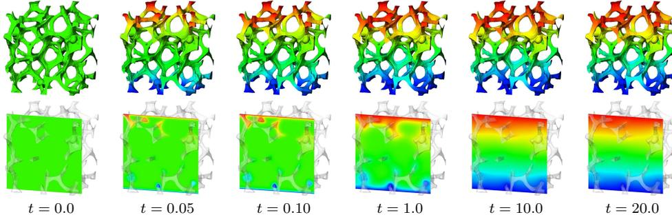
FIG. 6.4. Heat conduction simulation on an Al foam embedded in PMMA. Temperatures (194.65 K  $\rightarrow$  373.15 K) are visualized on the interface (top row) and on a slice through the composite material (bottom row). The temperature profiles for different times show that an almost steady state is reached much faster in the metal than in the plastic.
