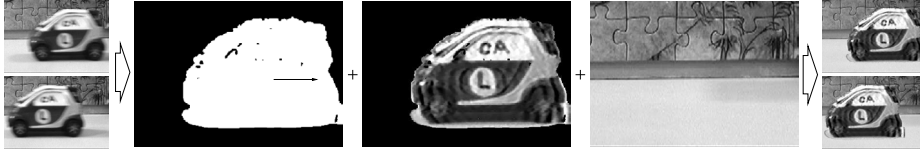
Fig. 17. From two real blurred frames (left), we automatically and simultaneously estimate the motion region, the motion vector and the image intensity of the foreground (middle). Based on this and the background intensity we reconstruct the two frames (right)
