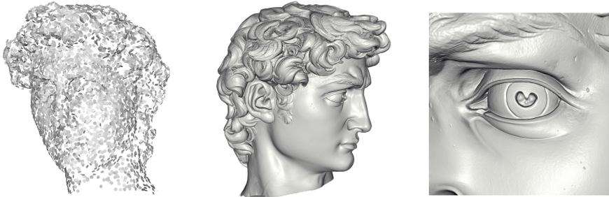
Figure 5: *Poisson Surface Reconstruction* proposed in [54] for high quality surface reconstruction from oriented points clouds. (Image courtesy of M. Kazhdan.)
