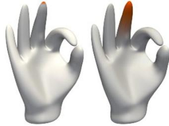
Figure 3: The equation  $\Delta_{\mathcal{S}}^2 u + u = f$  is solved on a surface using subdivision finite elements based on Loop subdivision with color coded  $f$  (left) and  $u$  (right) (Image courtesy of R. Perl).
