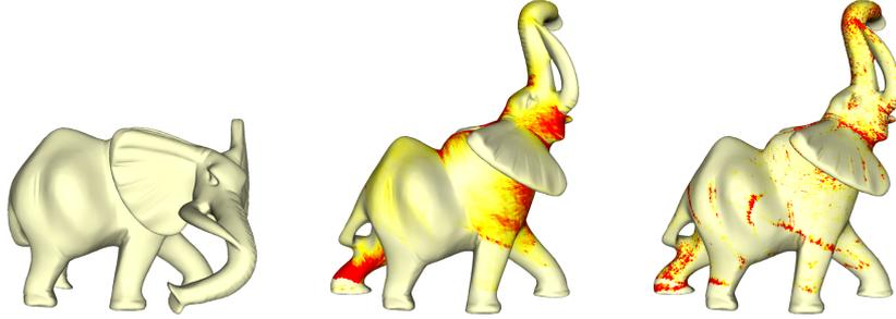
Figure 10: Two predominant types of deformation for a surface model (left) in the deformed configuration using a discrete geometry approach on triangular meshes: tangential stretching of shearing (middle, 0  $\rightarrow$  0.001) and normal bending (right, 0  $\rightarrow$  0.1).
