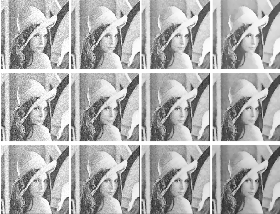
Figure 4.7 Non-linear diffusion solvers in graphics hardware and software; first row: adaptive software pre-conditioned conjugate gradient; second row: Jacobi solver in graphics hardware; third row: conjugate gradient solver in graphics hardware. The black borders are due to restrictions in handling of the boundary conditions in graphics hardware. The fine roundoff pattern in the images (electronic version only) is explained in the text (Section 4.1.4.2 on page 136).
