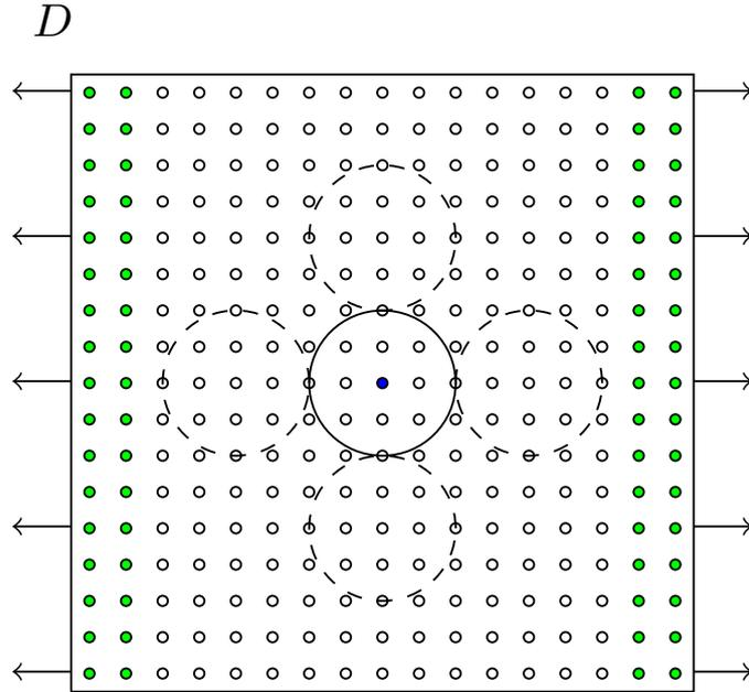
Figure 8: Cross section in  $x$ - $y$ -direction of the cube  $D$  centered at  $(1 \text{ m}, 1 \text{ m}, 1 \text{ m})^T$ . The green colored nodes indicates where the displacement of  $\pm 1 \text{ mm s}^{-1}$  is applied.
