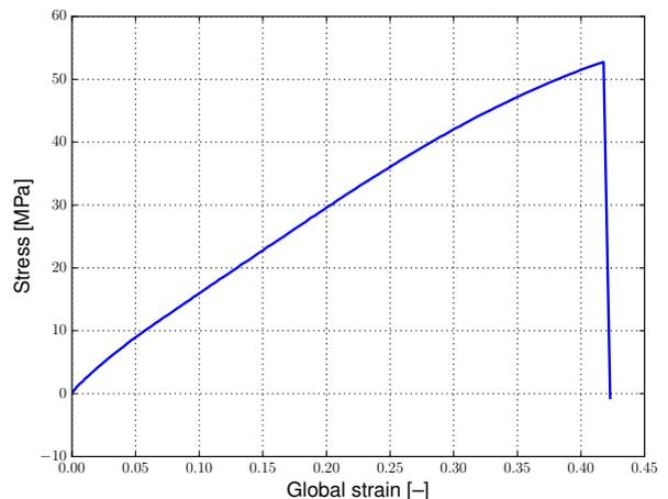
(b) The global strain vs. stress curve for PMMA.
