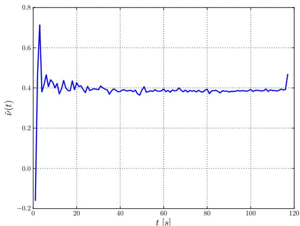
(a) The time-dependent Poisson ratio for PMMA.
