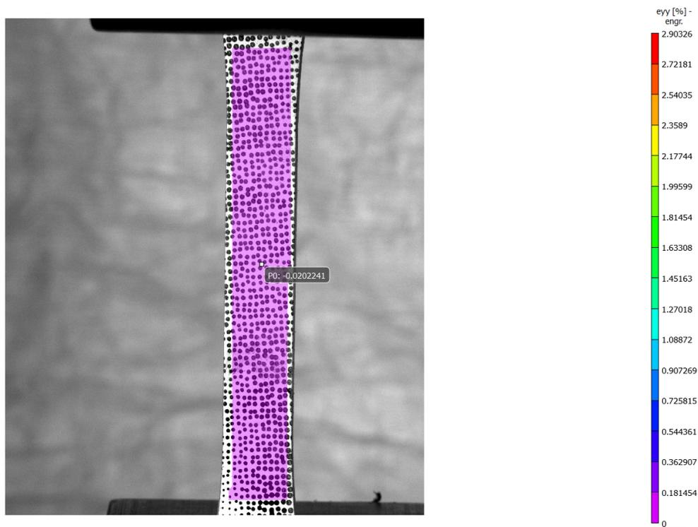
Figure 13: Extracted strain in  $y$ -direction of the experiment via digital image correlation
