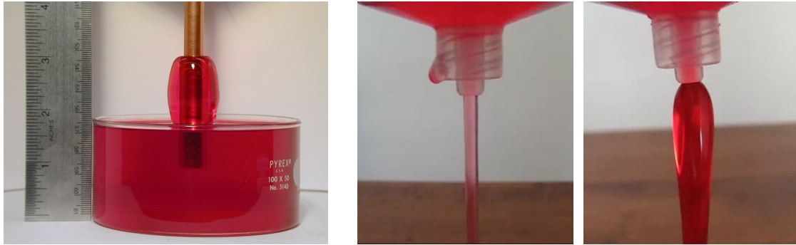
(a) Weissenberg effect (G. McKinley [48]). (b) Die swell in Newtonian and polymeric liquids (YouTube, Psidot [56]).
