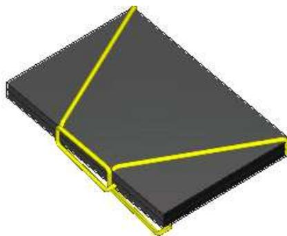
Fig. 8.14.: WiseTex model of the Non Crimp Fabric.
