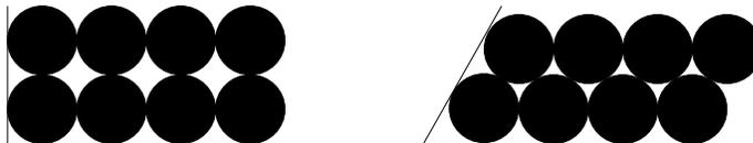
Fig. 7.1.: 2D cut of a packed bed of spheres with cubic packing (left) and rhombohedral packing (right).
