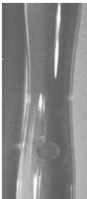
Figure 1.1.: Photo of a levitated droplet in a measurement device. The photo was taken applying an exposure time of 3 seconds to show the stability of the droplet. Provided by project B3, SFB 540.
