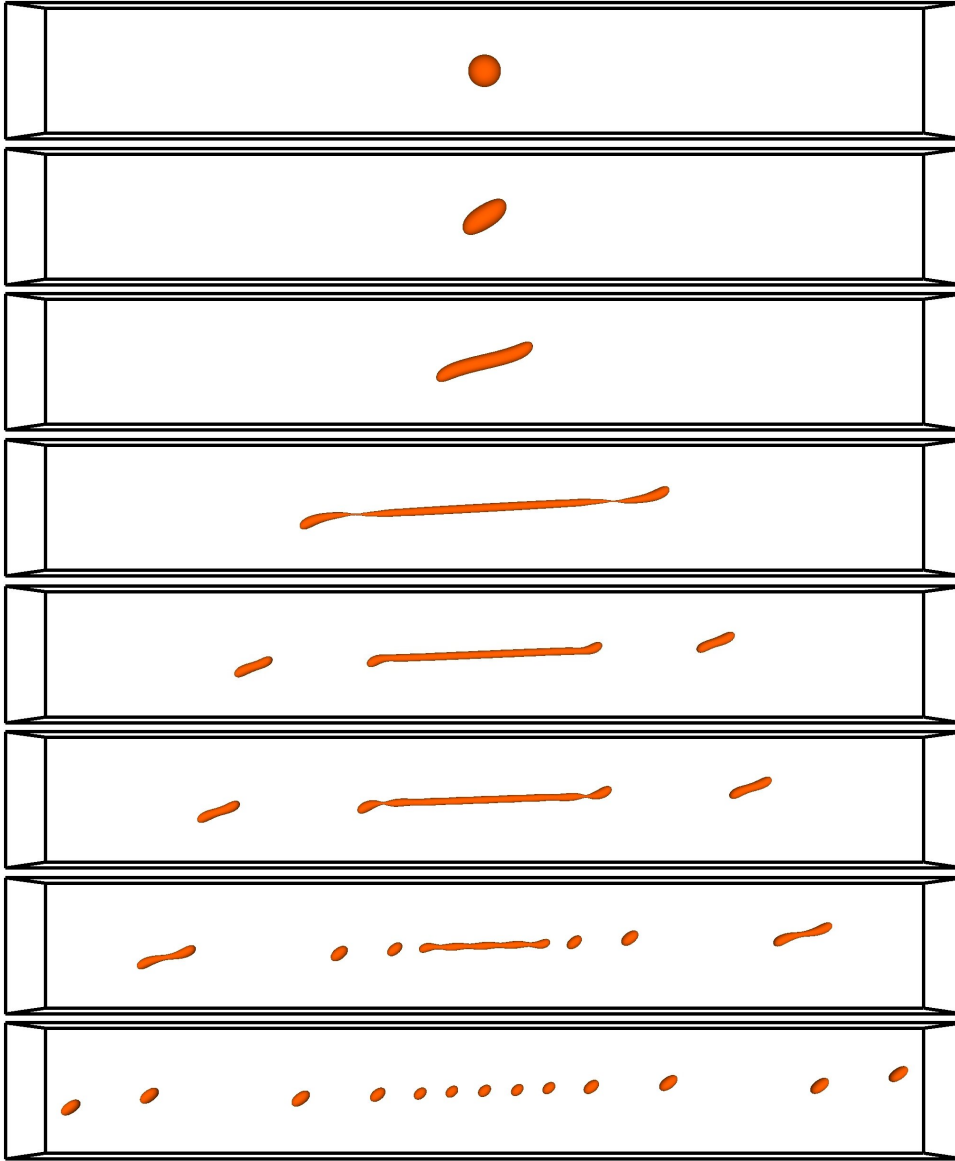
FIGURE 4.8. Instationary results obtained for the parameter setting (Ca, Re) = (0.1, 25) . Depicted are the configuration of the free surface at the times t = 0 , t = 178.8 , t = 238.8 , t = 330.0 , t = 358.8 , t = 373.2 , t = 394.8 , t = 418.8 (top to bottom). The simulation domain is 14 \times 1 \times 2 and the droplet has a radius of r = 0.25 . The mesh-width is (14/896, 1/64, 2/128) .
