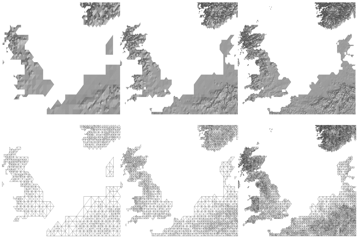
Figure 6: Adaptive triangulations and corresponding illumination shaded DEMs of the North Sea area based on the L_1 -norm without focus on coastlines.
