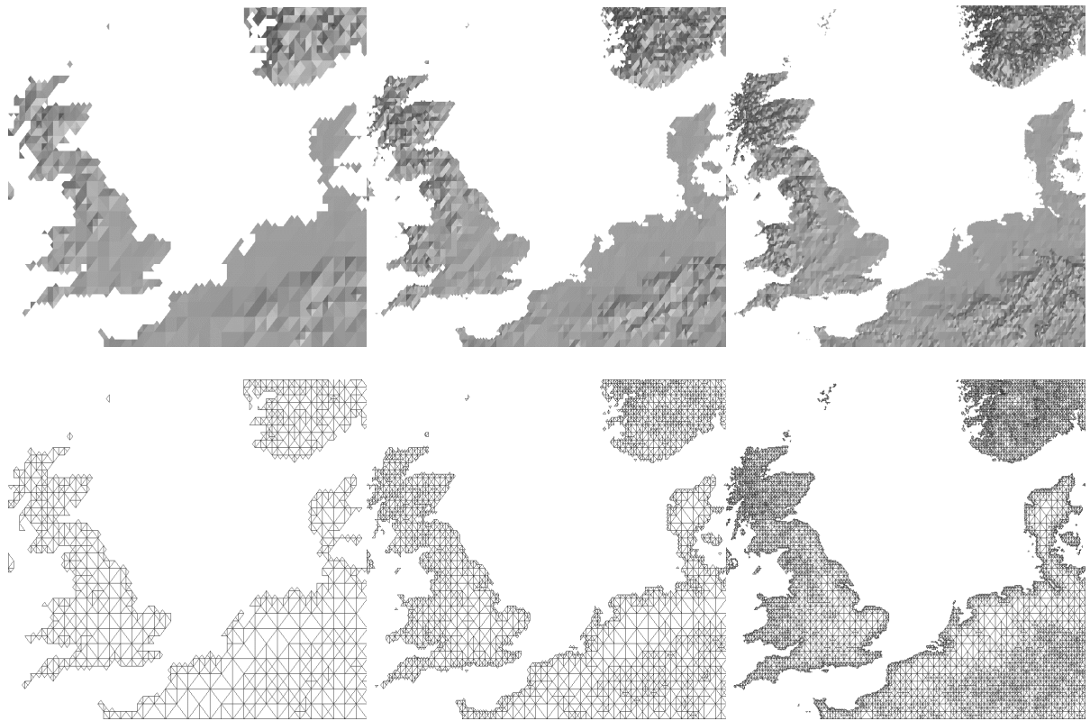
Figure 7: Adaptive triangulation and corresponding illumination shaded DEMs of the North Sea area based on the L_1 -norm with focus on coastlines.
