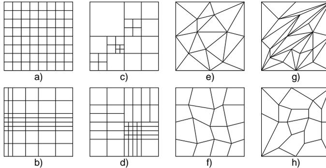
Figure 1: Examples for spatial decompositions used in DEMs.
