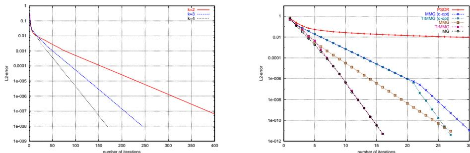
Figure 4: Iteration history of the projected Gauss–Seidel scheme (left) and of different MMG-variant based on piecewise quadratic,  $C^1$ -smooth B-spline basis functions (right).
