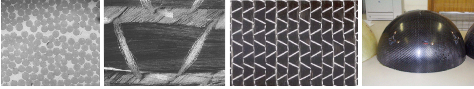
FIG. 1.1. A hierarchy of textile structures from left to right: the fibres ( a , 0.00001 m), the fabric unit cell ( b , 0.01 m), the composite unit cell ( c , 0.1 m), the composite part ( d , 1 m) [Pictures by courtesy of S.V. Lomov].
