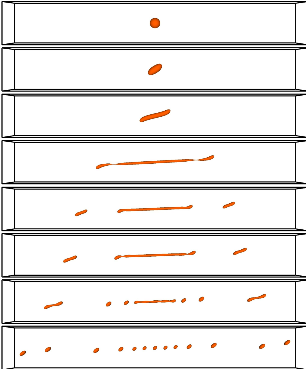
Figure 14. Instationary results obtained for the parameter setting (Ca, Re) = (0.1, 25) . Depicted are the configurations of the free surface at the dimensionless times t^* = 0 , t^* = 178.8 , t^* = 238.8 , t^* = 330.0 , t^* = 358.8 , t^* = 373.2 , t^* = 394.8 , t^* = 418.8 (top to bottom). The simulation domain is 14 \times 1 \times 2 and the droplet has a radius of r = 0.25 . The mesh-width is (14/896, 1/64, 2/128) .
