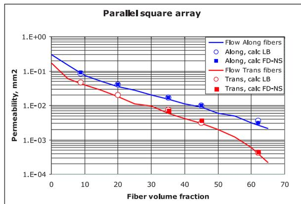
Fig. 3. Permeability of Parallel Square Arrays with different fiber volume fractions. Full lines: theoretical permeability; circles: Lattice-Boltzmann results; squares: Navier-Stokes results.
