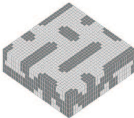
Fig. 2. Top,middle: A 2D-textile model and its first order approximation on the grid; bottom: 3D voxel geometry
