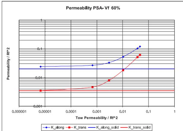
Fig. 4. Permeability of a Parallel Square Array with different local permeabilities
