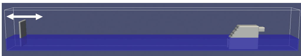
Fig. 5.4.1: Setup of the computational domain including the wavemaker (left) and the OWC Geometry (right) [Peuker, 2011].
