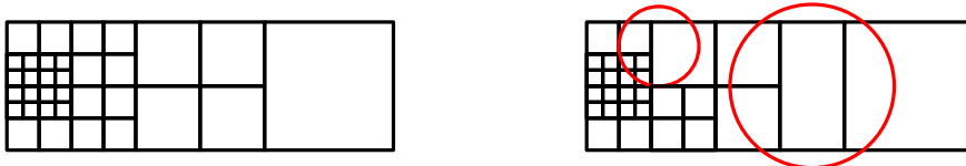
Figure 3. A one-irregular grid (left) and a grid containing several mistakes (right). Look for the edge with multiple ‘hanging’ nodes and for the rectangular shaped element, indicated by the labels.
