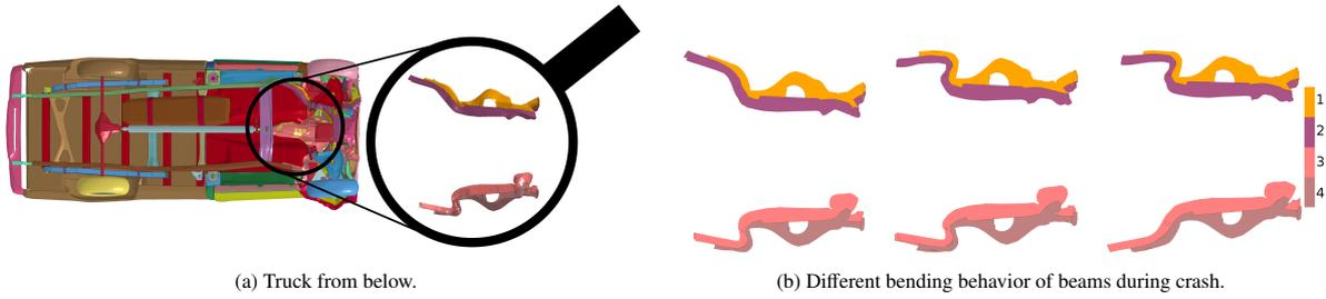
Fig. 2. We consider a Chevrolet C2500 pick-up truck as model problem. In (a) we show the truck from below at time step 17 (after the crash) and the position of beams nr. 1 to 4. In (b) the four essential beams at time  $t_{17}$  for three simulation runs. The color bar shows the labels of the beams (physical parts). A different bending behavior in each simulation run can be recognized.
