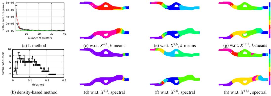
Fig. 3. Both, the L-method (a) and the density-based heuristic (b), estimate between 6 to 8 clusters. In (c)–(h) clustering of beams with *k*-means (top) and spectral clustering (bottom) for displacements (left to right) from  $t_3$  to  $t_4$ , from  $t_6$  to  $t_7$  and from  $t_1$  to  $t_{17}$ . The illustrations were performed using the FE model at time state  $t_1$ .
