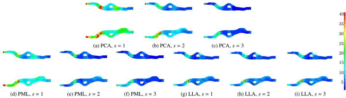
Fig. 4. Mean of the squared  $l_2$  errors of the reconstructed displacements over all test runs for the  $k$ -means clustering at the time steps  $t_i = 7$ ,  $t_j = 6$  for PCA, PML and LLA. The latent space dimension  $s$  increases from left to right. Values greater than 40 are colored red.
