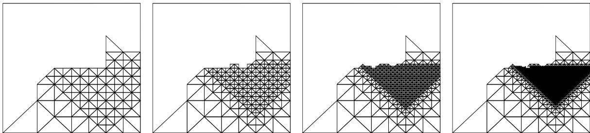
**Figure 11:** The culling metric  $\mu_{cull}$  based on the octagon distance for maximum levels of 8, 10, 12, and 14.
