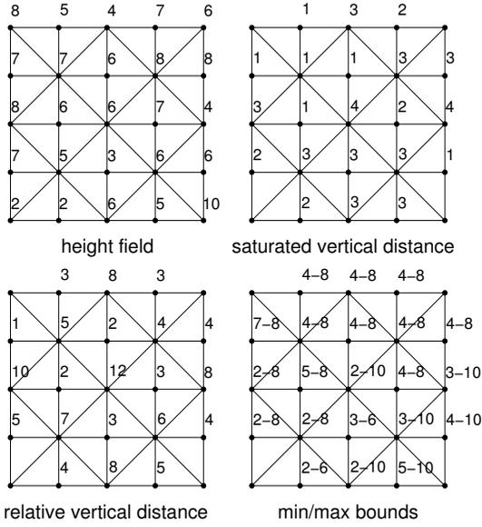
**Figure 2:** A few examples for the construction of saturated geometric distance metrics on a  $5 \times 5$  elevation grid.
