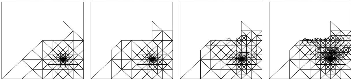
**Figure 12:** The combined metric  $\mu = \mu_{geo} \cdot \mu_{dist} \cdot \mu_{cull}$  for thresholds of 1, 0.1, 0.01, and 0.001.
