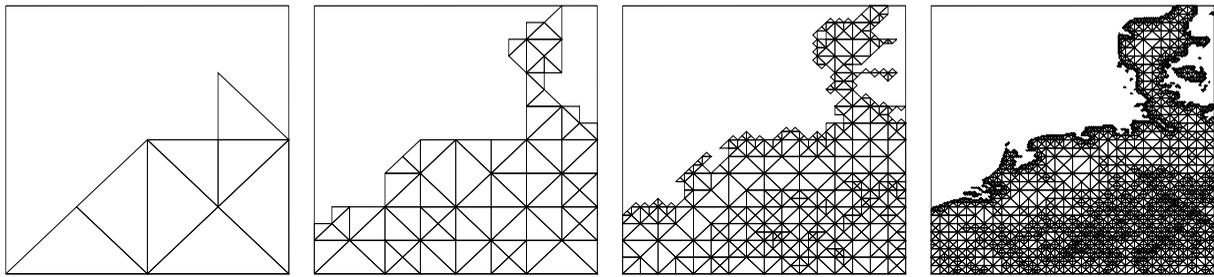
**Figure 9:** The geometric distance metric  $\mu_{geo}$  for thresholds of 1, 0.1, 0.01, and 0.001.
