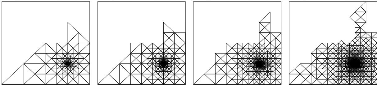
**Figure 10:** The distance metric  $\mu_{dist}$  based on the octagon distance for thresholds of 1, 0.1, 0.01, and 0.001.
