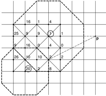
**Figure 7:** In this example we show the squared octagon distances (in order to avoid square roots) from the point  $\mathbf{p}$  to the refinement vertices of a  $5 \times 5$  grid. The distance between the grid points is 1. The corresponding octagons of the two encircled vertices are shown dashed.
