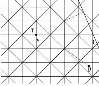
**Figure 5:** The octagon distance from a point  $\mathbf{p}$  to a triangle  $T$  is the distance of  $\mathbf{p}$  to its corresponding octagon  $o_l(T)$ . Similarly, the octagon distance from a line  $\mathbf{l}$  to the triangle is the distance between  $\mathbf{l}$  and its octagon  $o_l(T)$ .
