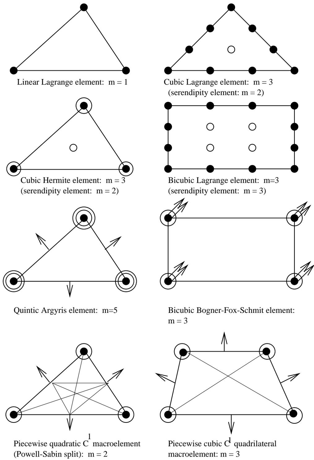
Figure 6: Local interpolation problems for some FE types
